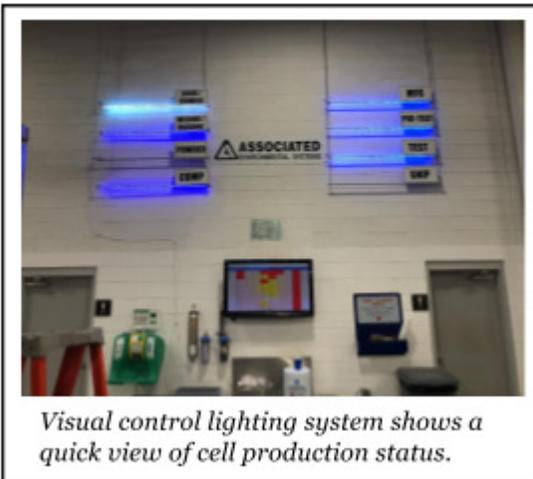
One key change was the implementation of a Visual Control System. Lights installed above each cell give a visual representation of the status of the operation. A red light indicates the process has a work-stopping issue and a white light indicates the operation is proceeding normally. Other colors have been implemented to signify various production statuses. All lights can be seen at a glance throughout the facility.
